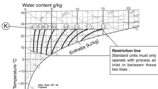
The dehumidifying capacity is estimated as the nominal capacity from the table (on the reverse side of this document), multiplied by the factor (K) from the correction diagram. For inlet conditions of 20°C/60%RH, the data given is correct for all models. For all other inlet conditions, the correction factor can vary ±10% for different size units. The dry air temperature for Frigosorb is calculated with help from the below formula and with the K-factor from the diagram for Frigosorb.
