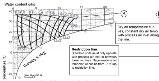
The dehumidifying capacity is estimated as the nominal capacity from the table (on the reverse side of this document), multiplied by the factor (K) from the correction diagram. The dry air temperature for Econosorb is calculated from the above diagrams.
